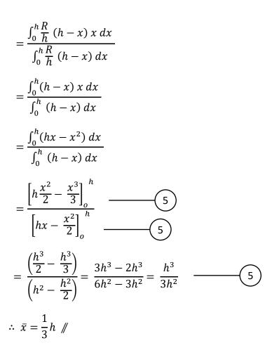
Entire cone is symmetry about OX axis.  $\therefore$  The centre of mass of entire cone is on OX.
