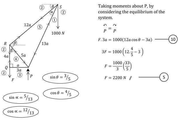
Other than the reaction at P, the other two forces acting on the system are - F vertical force at Q and 1000 N at S only.
