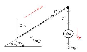
F = ma 3m  $4 \Rightarrow 3mg - T' = 3mF$  5  $7 \Rightarrow T' - 2mg\cos(\pi/3) = 2mF$  2mg = 5mF  $F = \frac{2}{5}g \#$
