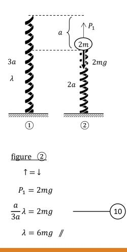
In this incident there exist two S.H.M.S with masses  $2m \& m \therefore We$ have to show that there exist two S.H.M & have to find  $\omega_1 \& \omega_2$ W.R.T. those S.H.M. And also the two centres.
